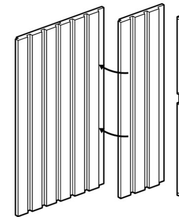
Always lay the panels starting from the left and then moving right and starting from the bottom, moving up.
