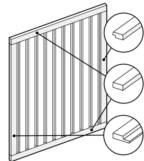
To finish the wall, use the system trims, which, like panels, are mounted with adhesive. For each of the panel types, you can choose the right and left trims, while the universal trim will allow you to finish the top and bottom of the wall.
