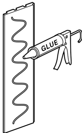
Apply adhesive on the back of the panel in the shape of the letter „S“, then attach the panel to the wall.
