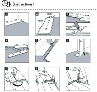
Use a sufficient number of wedges to maintain the gap. The boards should preferably be laid in the direction of incoming light. In small, narrow areas (e. g. hallways) we recommend that installation follows the length of the room.
