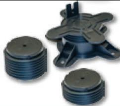
We suggest that you use our **decking base** as the weight-bearing surface for the underconstruction. The distance from the centre should be 40 to 60 cm.
